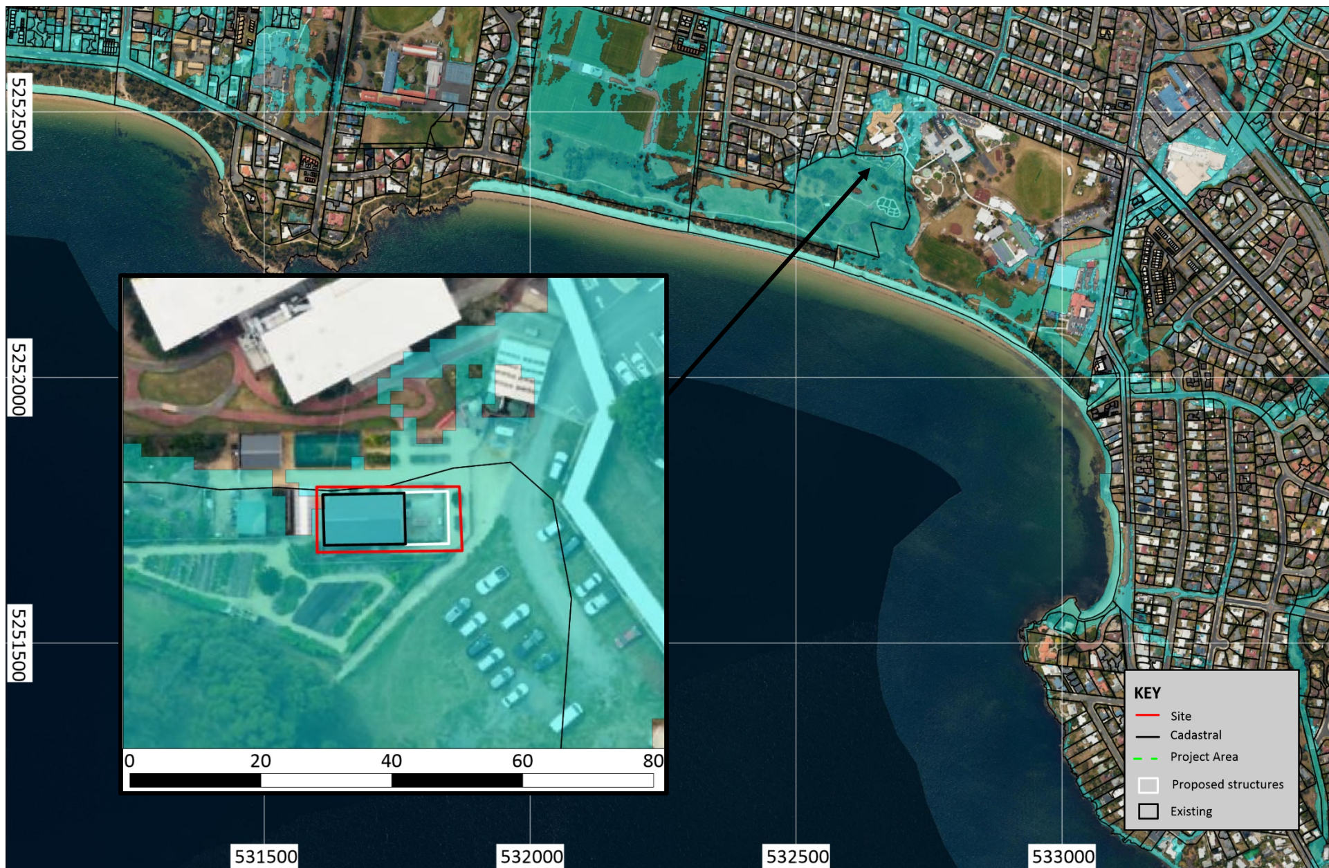
Map 7 Flood prone areas overlay – 1% AEP inundation mapping
