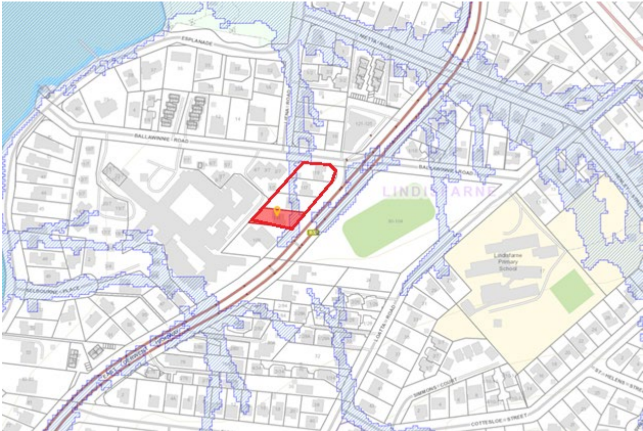
Figure 4 – Clarence City Council 1% AEP Flood Mapping (Source: ccc.tas.gov.au )
