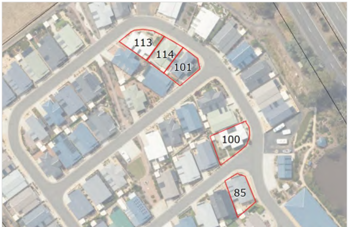
Figure 14: Established dwellings with dual frontage and reduced front/rear boundary setbacks (source: www.thelist.tas.gov.au © State of Tasmania)
