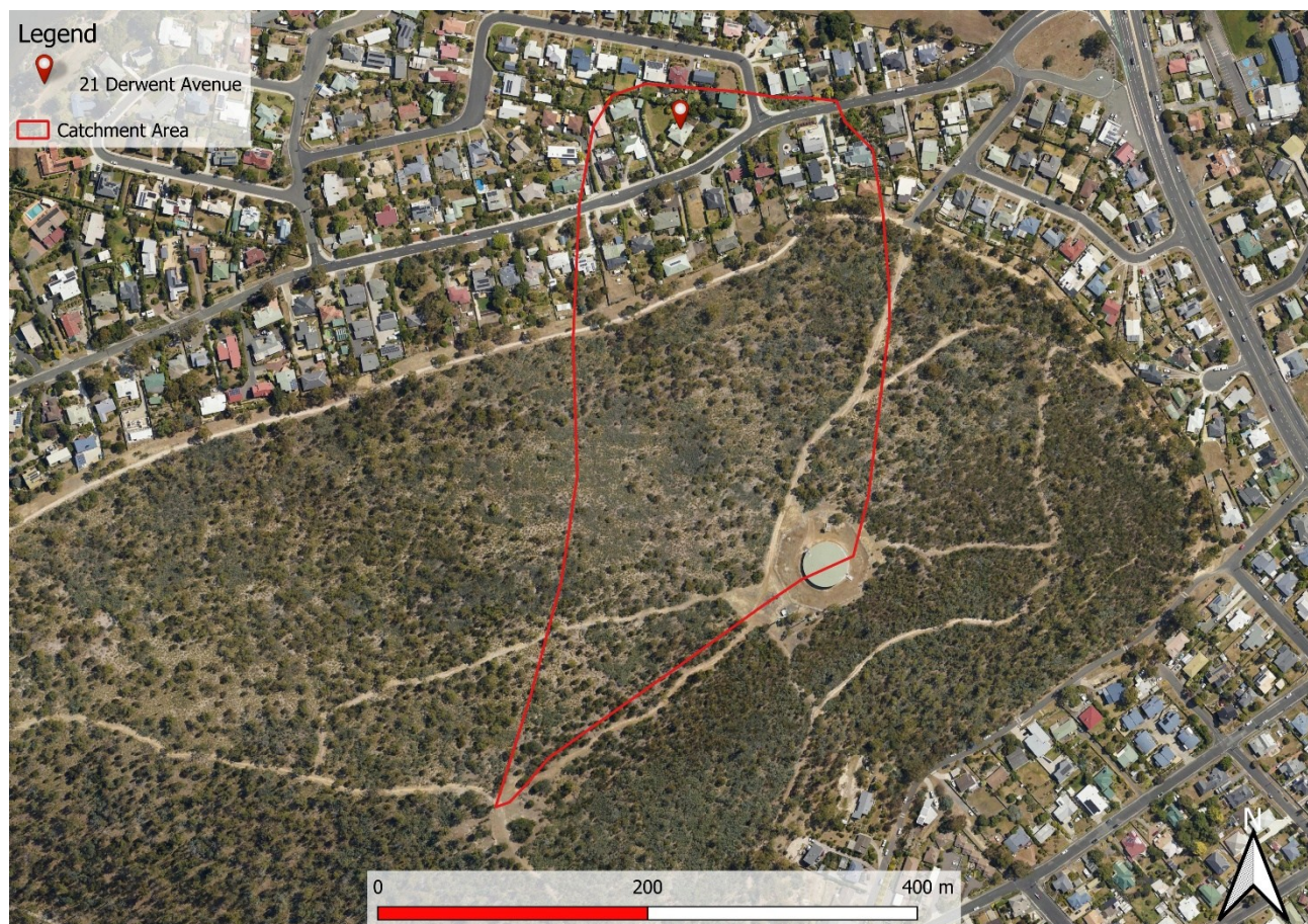
Figure 1. Contributing Catchment for 21 Derwent Avenue, Geilston Bay
