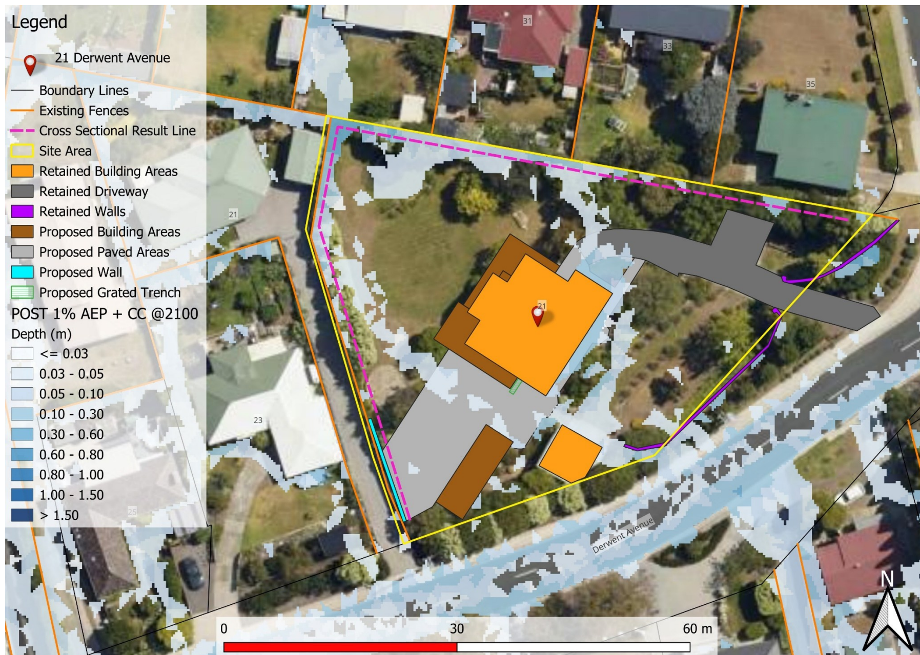
Figure 5. Post Development 1% + CC Flood Depth and Extents
