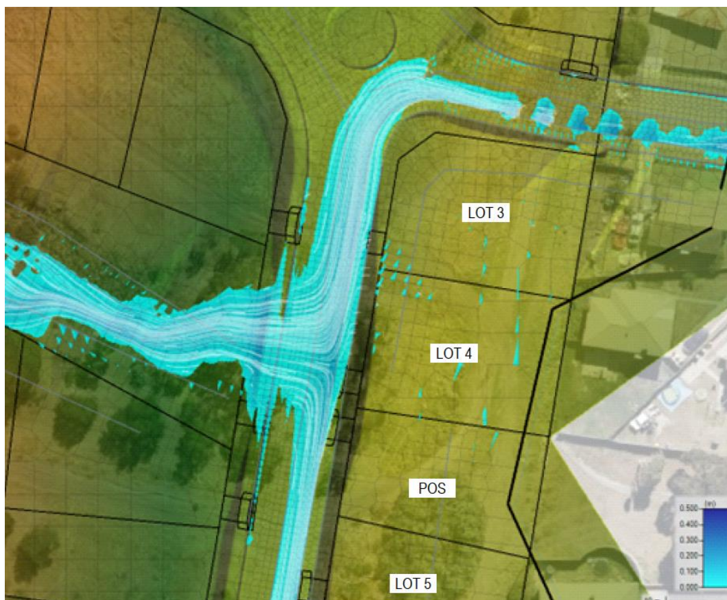
Figure 8 - Flow directional arrows across bottom roadway.
