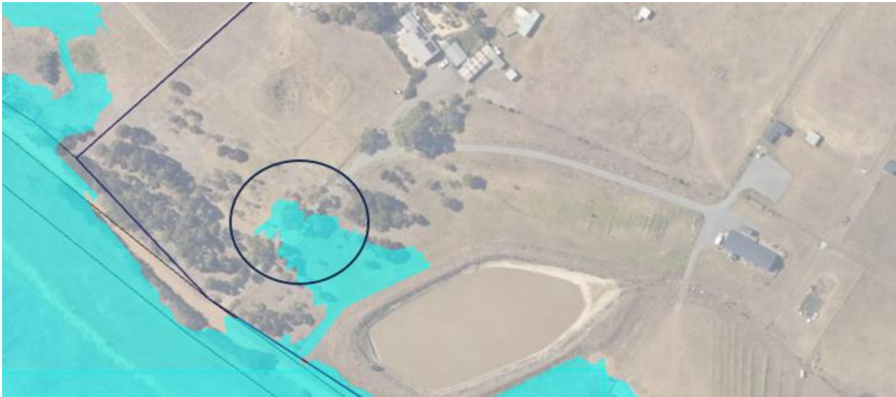
Figure 16: The internal roadway crosses a low coastal inundation hazard area.
